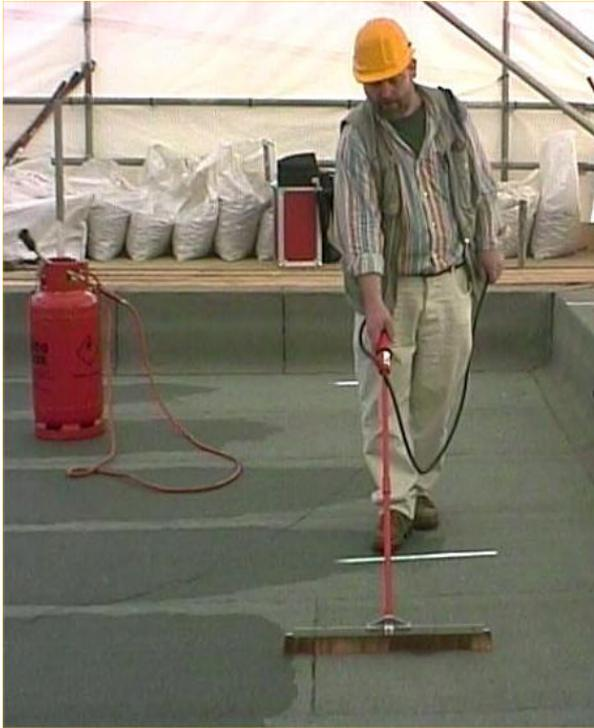
**Buckleys, specialist designers and manufacturers of High Voltage Test Equipment, have created “Roofing Test Kits” suitable for locating leaks in roof membranes. Damage can be caused by tradesmen working on the roof area, whether the structure is old or new. The problem is to find the faults which can be the size of a pinhole and invisible to the naked eye.**
